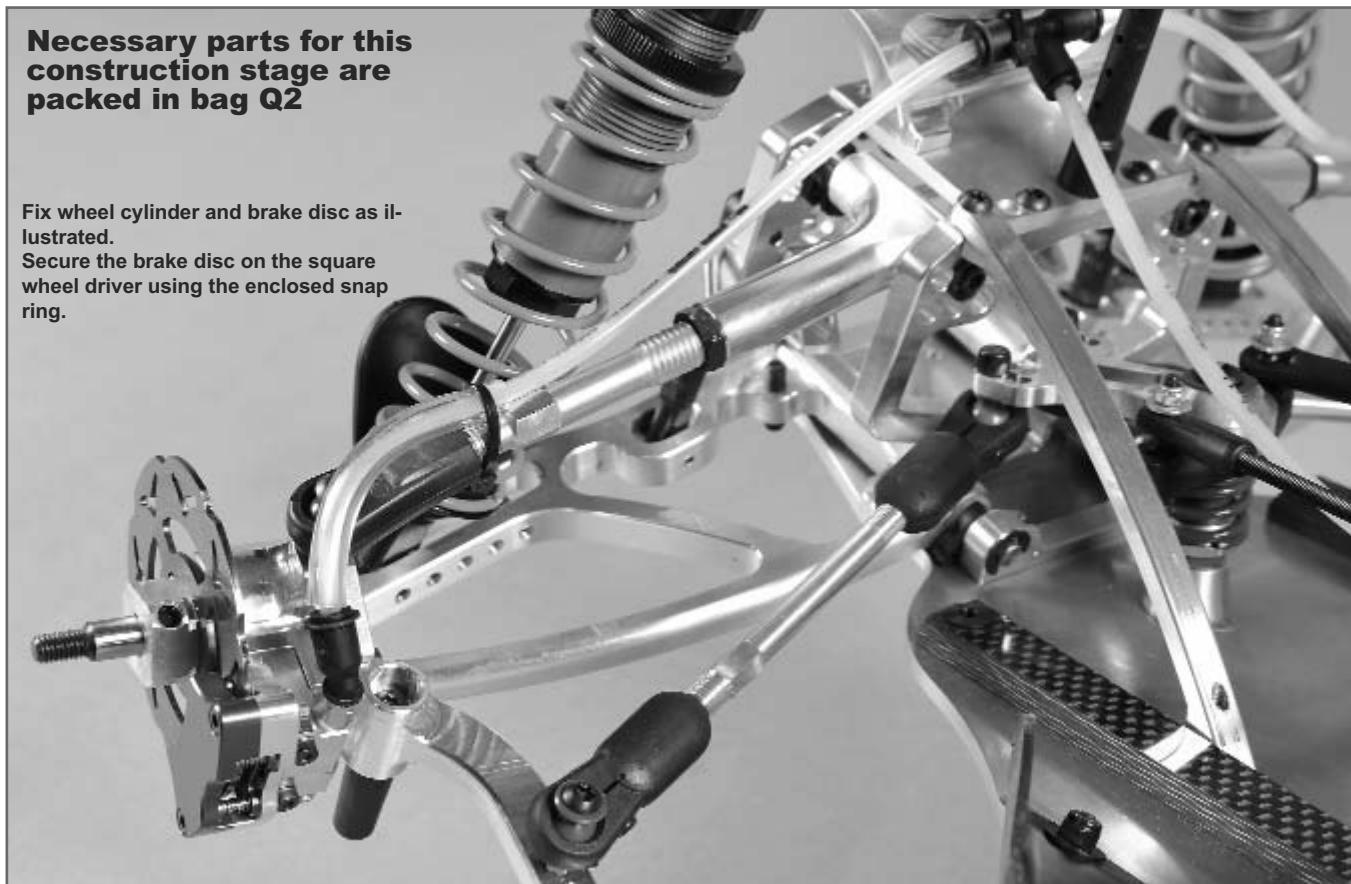
Fix the protective hoses on the brake tubes and place them as illustrated. Mount the snap rings at the connections and T-pieces. Make sure the brake tubes are not in close contact to hot vehicle components or sharp edges.
