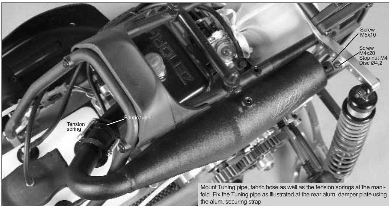
Mount Tuning pipe, fabric hose as well as the tension springs at the manifold. Fix the Tuning pipe as illustrated at the rear alum. damper plate using the alum. securing strap.
